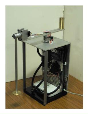
Rotary Inverted Pendulum System
