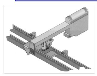
Fast Component Mounter Placement Module
