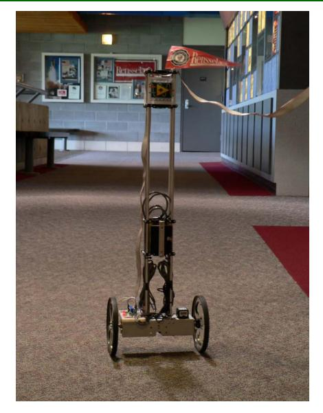
RPI Mechatronics Balancing Robot
